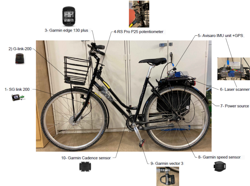
Figure 3. The instrumented bicycle used during the experiment. The numbers represent the different sensors mounted on the bicycle are described as follows. 1. SG-LINK-200-OEM + Hall Effect Sensor from Alliantech was used to count the number of rotations per minute (RPM) for the front wheel in order to calculate its angular velocity. The sampling rate was set to 250 Hz. 2. G-link-200 Triaxial accelerometer from AlianTeck is a wireless 3-axis accelerometer with \pm 2 to \pm 40 g measurement range. The sampling rate is up to 4096 Hz. 3. GPS (Global Positioning System): Edge 130 plus from Garmin that includes: GPS, GLONASS, and GALILEO systems to detect position in real time. 4. P25 wire-wound potentiometer from RS Pro, it is connected with specially designed cogs and attached to the handlebar to measure the steering angle. The sampling rate is 100 Hz. 5. Inertial Measurement Unit (IMU) unit+ WLAN “Shell” 4.0 Data Logger: from Avisaro, was used as a data logger with a 6 DOF IMU unit (3 axis acceleration/3 axis gyro). The IMU sampling rate was set to 100 Hz. 6. OY1P303P0189 laser scanner, from Wenglor, was used for the continuous measuring of the distance between the top of the rear seat and the road surface. The sampling rate is 30 Hz. 7. K2 powerbank, from PowerOak, was used as a battery to provide power to the laser scanner and the data logger. 8. Speed sensor 2, from Garmin, is a wireless sensor that gives longitudinal velocity. 9. Vector 3 power meter pedals from Garmin provides dual-sensing on both pedals. 10. Cadence sensor 2 from Garmin, was fastened to the left-side crank arm to measure pedal strokes per minute.
